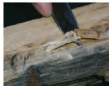
Pick test on decayed wood—brash break
