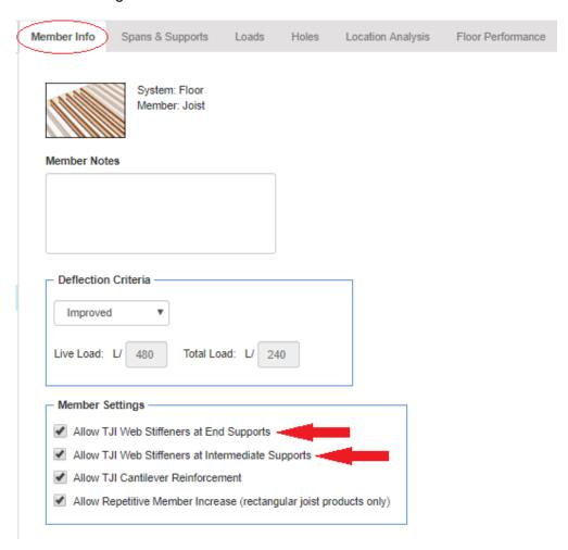
In summary, web stiffeners are not a means for vertical load transfer around a TJI® joist, but rather increase the allowable reaction of a TJI® joist or provide lateral stability. Please review your structural details pages and/or the construction or placement plans to ensure that end bearing details reflect the proper use of web stiffeners. Refer to TJI® 110, 210, 230, 360, and 560 Specifiers Guide (TJ-4000) or the Trus Joist® Framer's Pocket Guide for installation details.
