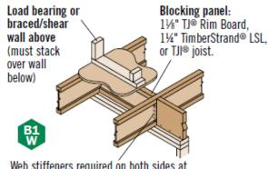
Web stiffeners required on both sides at B1W ONLY. See footnote 1 under span tables.
