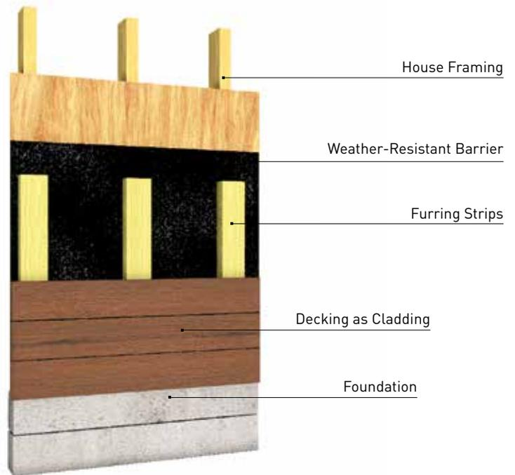
Cladding deck boards use a square shouldered profile and are 1" x 5½"
