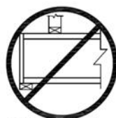
Uniform loads only--no offset bearing walls
