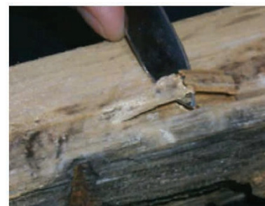
Pick test on decayed wood—brash break
