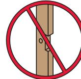
DO NOT cut a notch and a hole in the same cross section
