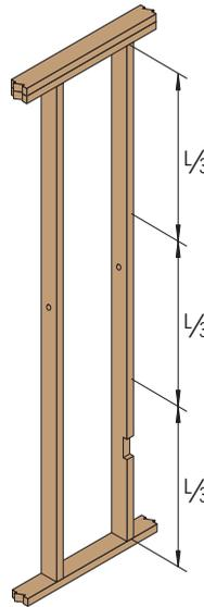
When used in conventional construction applications, both 2x4 and 2x6 TimberStrand® LSL studs may be drilled or notched in accordance with IRC Section R602.6.
