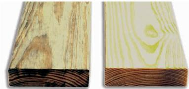
**Untreated lumber (at left) exposed to moisture can become a costly problem. Lumber protected with an effective anti-mold and anti-sapstain solution (at right) combined with good inventory control practices addresses this problem.**
