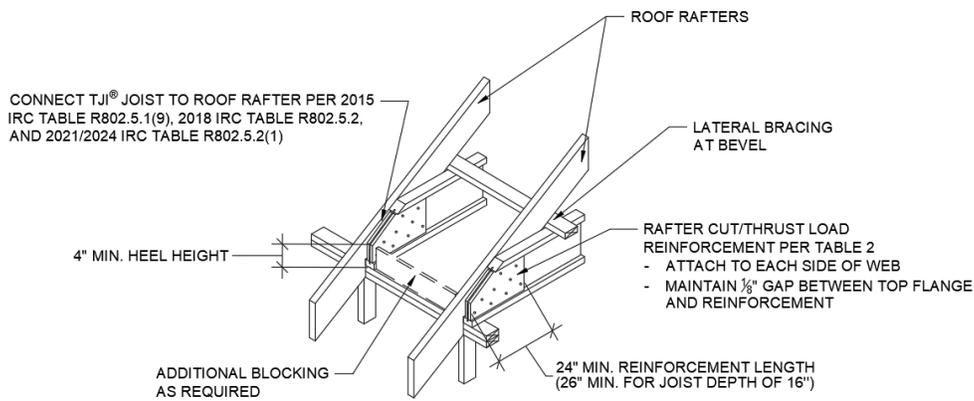
**TABLE 2: RAFTER CUT/THRUST LOAD REINFORCEMENT**
