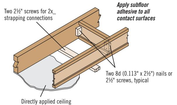
**PB1** When specified in design software or layouts, one of the above bracing options is required
