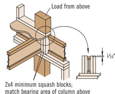
**CS** *Use 2x4 minimum squash blocks to transfer load around TJI® joist*
