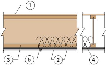
1. 48/24 tongue-and-groove, span-rated sheathing (Exposure 1), glued with a subfloor adhesive and nailed.
