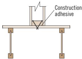
Nail interior partitions to the joists when possible. If the wall can be nailed only to the floor panel, run a bead of adhesive\* under the wall and either cross nail, nail through and clinch tight, or screw tightly into the wall from below.
