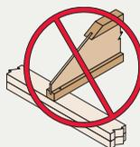
DO NOT bevel cut joist beyond inside face of wall.
