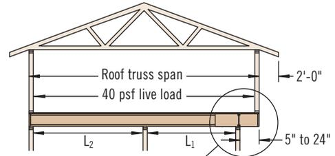
TJI® joists may be cantilevered 5" to 24" when supporting roof load, assuming:
