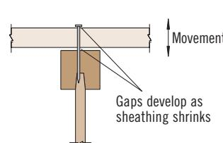
Keep building materials dry, and properly glue floor panels to the joists. Panels that become excessively wet during construction shrink as they dry. This shrinkage may leave gaps that allow the panel to move when stepped on.
