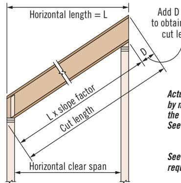
Actual cut length can be approximated by multiplying the horizontal length by the slope factor and adding the D factor. See tables below.
