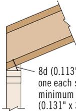
8d (0.113" x 2½") nail, one each side, 1½" minimum from end. Use (0.131" x 3") nails with TJI® 560D joists.
