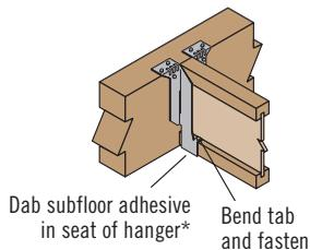
Seat the joist tight to the bottom of the hanger. When using hangers with tabs, bend the flange tabs over and nail to the TJI® joist bottom flange. Placing a dab of subfloor adhesive\* in the seat of the hanger prior to installing the joist can reduce squeaks.
