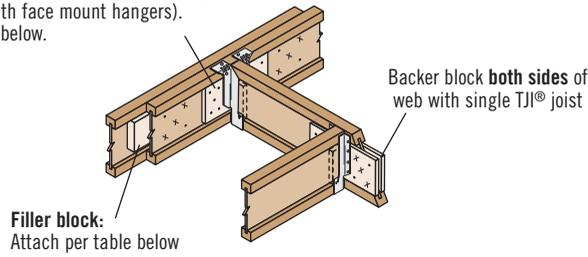
**H2** With top mount hangers, backer block required only for factored downward loads exceeding 395 lbs or for uplift conditions
