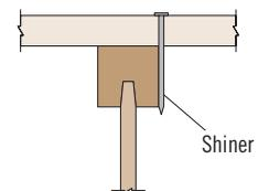
Exercise care when nailing. Nails that barely hit the joists (shiners) do not hold the panel tight to the joist and should be removed. If left in, the nails will rub against the side of the joist when the panel deflects.
