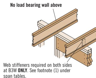
**B3** **B3W** *Blocking panels may be required with braced/shear walls above or below—see detail B1*
