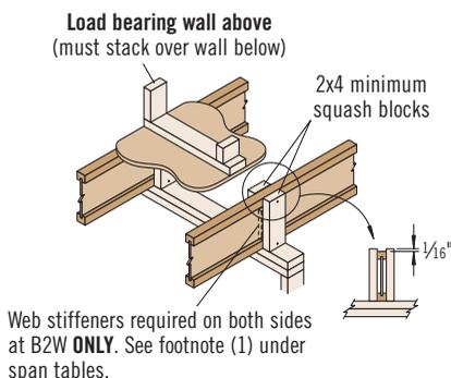
**B2** **B2W** *Blocking panels may be required with braced/shear walls above or below—see detail B1*
