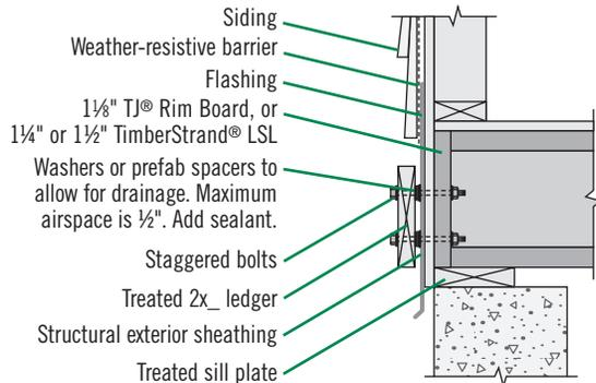
Maintain 2" distance (minimum) from edge of ledger to edge of fastener. Stagger bolts.
