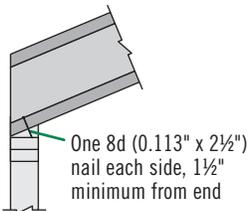
*When slope exceeds ¼:12, a beveled bearing plate, variable slope seat connector, or birdsmouth cut (at low end of joist only) is required.*
