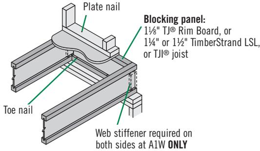
**A1** **A1 W** Attach blocking per A3.1 in rim board installation table above
