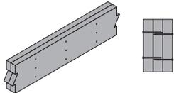
**L6** Multiple pieces can be nailed or bolted together, up to a maximum width of 7"
