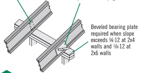
**R7** **R7W** **R7S** R7S is required for slopes greater than 3:12.
