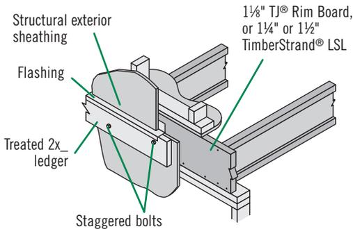
**LA** Corrosion-resistant fasteners required for wet-service applications
