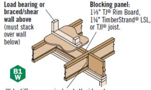
Web stiffeners required on both sides at B1W **ONLY**. See footnote 1 under span tables.
