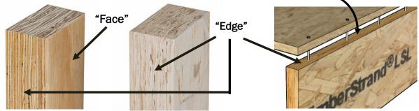
TimberStrand® LSL may permit closer fastener spacing (and more rows of fasteners) than Microllam® LVL in the "narrow edge" orientation. The excerpt below is from Table 2 from Trus Joist Technical Bulletin <u>TB-206</u> – Fastener Spacing in Weyerhaeuser ELP.
